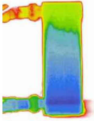
6.17b Thermo camera picture of refrigerant distribution in a BPHE with distribution device.
