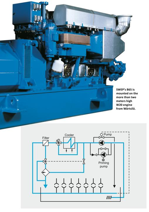
All W20 engines are equipped with a complete lube oil system, i.e. an mechanically driven main pump, electrically driven prelubricating pump, cooler, full flow filter and centrifugal filter.
