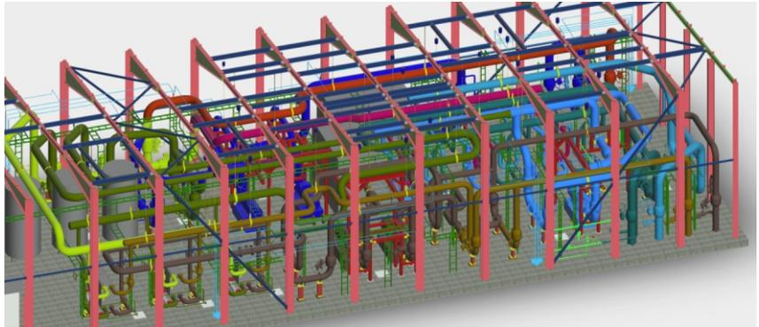
B649 BPHEs are connected between the power plant and the district heating network in Høje-Taastup. Alongside, regular gasket heat exchangers act as intermediate units between the thermal storage and the SWEP units.
