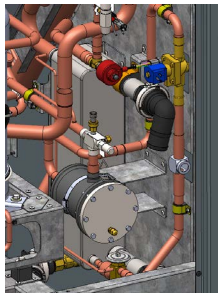
Screenshot from 3-D CAD model of the Laser Chiller showing a Q80ASx60 SWEP All-Stainless brazed plate heat exchanger.
