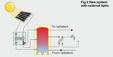
Low-flow variants of the two-circuit system maintain different temperature zones in the water tank, supplying heating and sanitary water separately.
